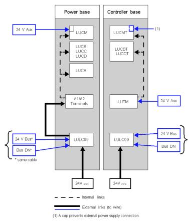
24V Bus = Communication module power supply (V+ and V-)
