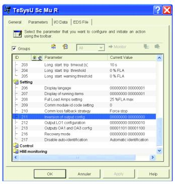
When you select a parameter (selected parameters are highlighted in blue), you can press the keys Ctrl + H to access a Help screen that provides the register number:
