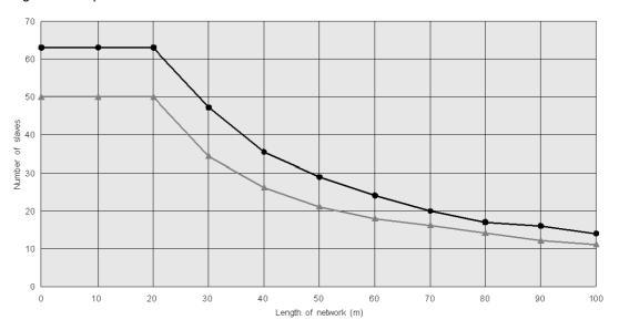
The number of TeSys U devices connected on the DeviceNet network can be increased if necessary by using a second DeviceNet power supply.
